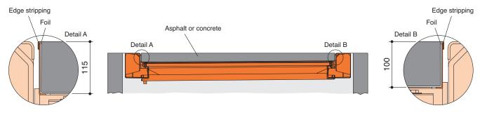
Before filling the trough with concrete or asphalt, edge stripping must be placed around the edges on site. Before filling, the trough must be lined with a water-<u>im</u>permeable foil by a specialist company on site. Dimensions rounded.
