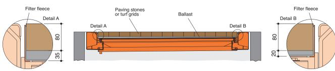
Before paving, the trough must be lined with a water-<u>permeable</u> filter fleece by a specialist company on site. Dimensions rounded.
