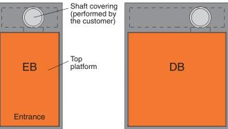
Serial system (EB and DB can be combined)
