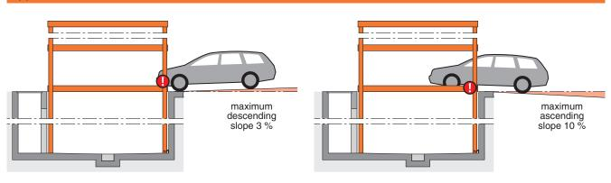
The illustrated maximum approach angles must not be exceeded. Incorrect approach angles will cause serious maneouvring & positioning problems on the parking system for which the local agency of KLAUS Multiparking accepts no responsibility.
