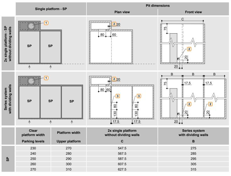
1 A shaft cover must be provided (to be provided by the customer).
