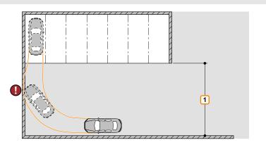
All side walls must be at a right angle. Deviation max. 1 cm!
